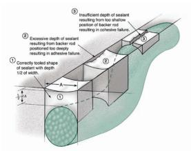
**NOTE:** Joints expected to withstand hydrostatic or shear forces must have a width to depth ratio of 1:1.
